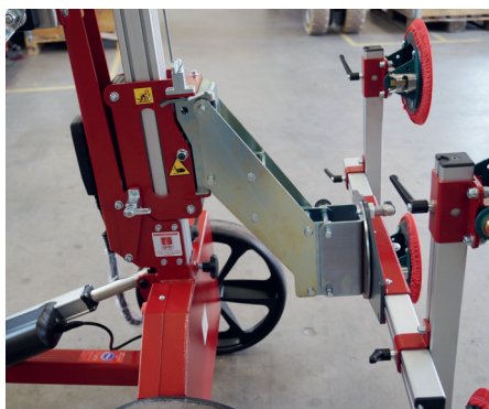
The extension diagonally downwards enables narrow discs to be accommodated
