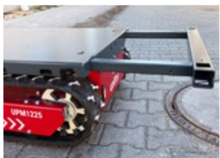
Extendable struts on both sides to extend the loading platform.
